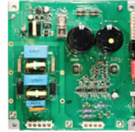
EPC Control Board
